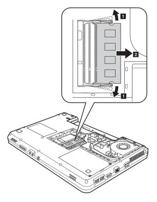
**7** Insert the notched end of the DIMM into the socket.
